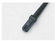
MTRJ is a duplex connector with both fibers in a single polymer ferrule. It uses pins for alignment and has male and female versions
